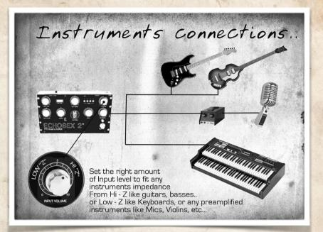
The Echosex 2° T7E let you use a variety of instruments both in low or high impedance, thanks to its Input Level Control (3) from a Guitar with single coils pickups to a Line level Keyboard, or any preamplified instrument directly in its Input (5) just by setting in the right way the Input volume. This is very important also for general connections of the machine in any situation like an Fx loop, a mixing console as described in the next chapter.
