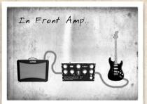
The Echosex 2° T7E is designed to be used even in front of an amplifier, its tube buffered out perfectly fit any quitar, bass, or organ amplifier. The most important thing is to set the Input Level, to fit the High impedance signal of your guitar or bass. In this configuration, our suggestion is to put the Echosex at the end of your chain, or at least after OD/Dist. pedals, to obtain the best performances.
