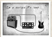
Connect your Echosex 2° T7E to the Ex Loop of your amplifier it's very simple use two mono jack cables, input to send, Main output to return. Very Important is to set in the right way the input Level, as the level of your preamp output (send) is very higher than a guitar signal, so you will have to set the Input control at a lower value. Help yourself with the Magic Eye to see when it's ok. Running into a loop, let you add beautiful, lushy carpets of sound both to your clean or Lead sounds.
