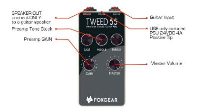
24VDC 4A (positive TIP) Power In **Power out** 55W RMS @4Ohm max 3%THD Consumption 2,5A >100K Ohm **Input Impedance Speaker Output Impedance** 4/8/16 Ohm S/N ratio <90db Larghezza (Width) 60mm. (2,3") Lunghezza (Length) 120mm. (4,7") Altezza (Height) 30mm. (1,1") Peso (Weight) 0,2Kg. (0,4lbs)
